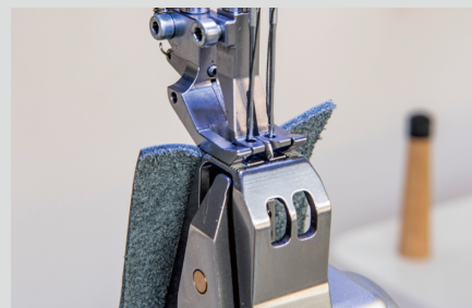
三同步送料系统，送料稳定精准。 Triple synchronous feeding system ensures stable and precise feeding.
