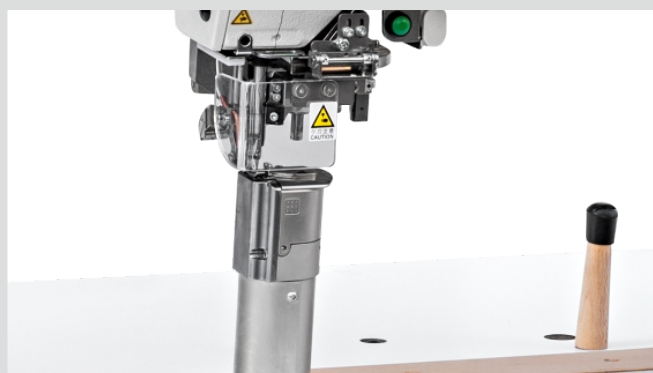
压脚、底牙、机针三同步送料，保证送料精准稳定 The three synchronous feeding of presser foot, bottom teeth, and machine needle ensures precise and stable feeding.
